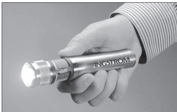
Figure 5. Angstrom Power has implemented its direct hydrogen fuel cell technology in products such as the A2 micro hydrogen™ fuel cell flashlight. Running on hydrogen stored in the handle and air from the environment, the 1 W LED flashlight delivers a continuous runtime of more than 24 h on a single charge of hydrogen.
